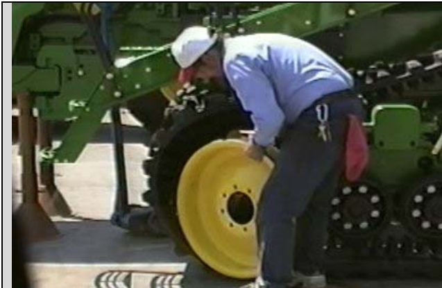
Front Idler Removal (John Deere)
