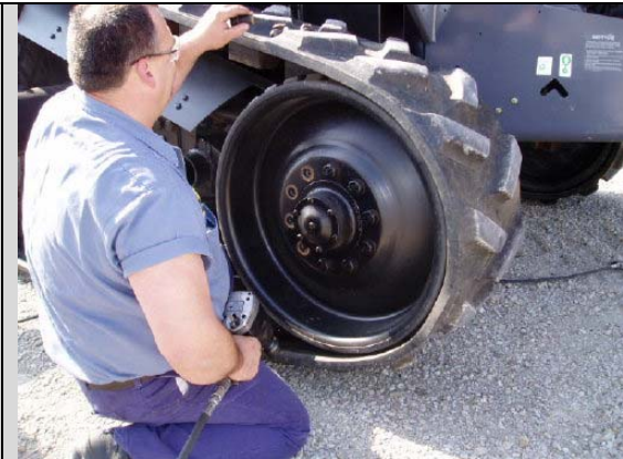
Front Idler Removal (Caterpillar 35/45/55)
