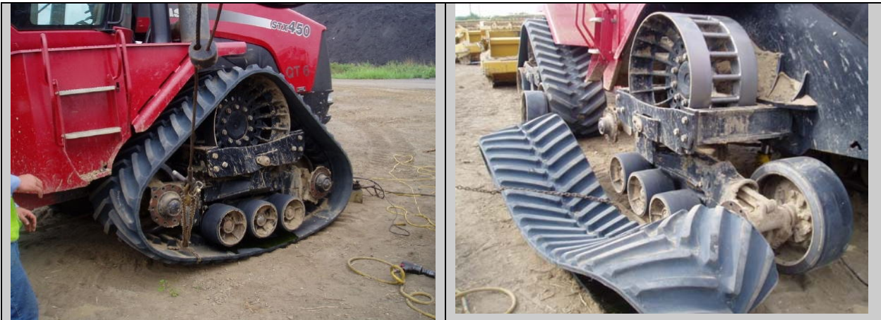
Using a boom truck to work track off the drivewheel and rear idler simultaneously
