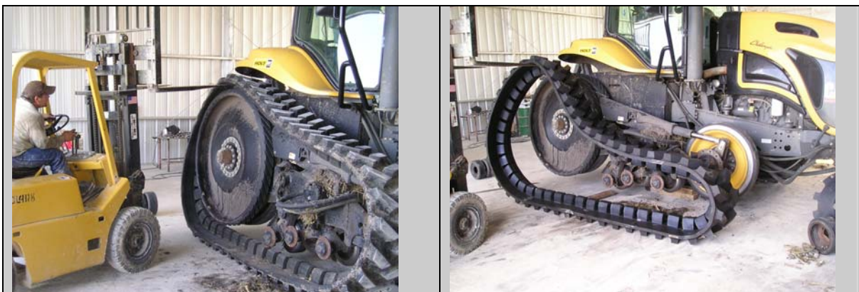
Using forklift to remove track
