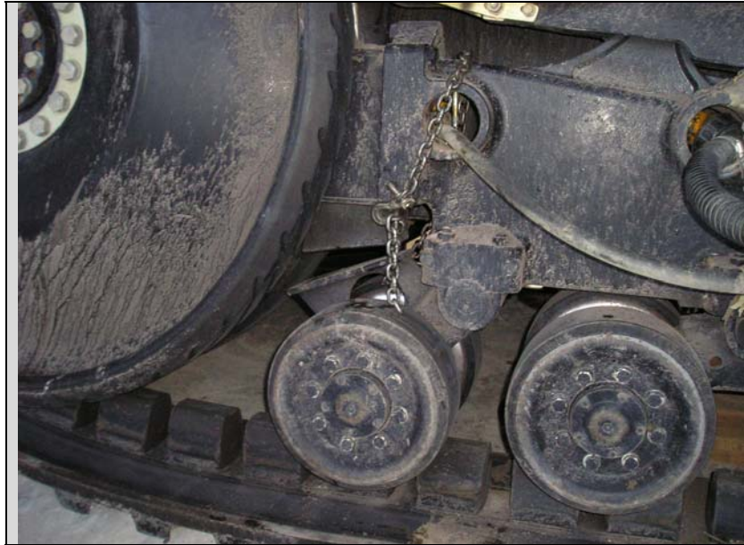
MT700 Only: Rear Midroller Supported
