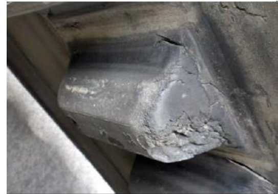
Typical Drive Lug Mid-Life Wear
